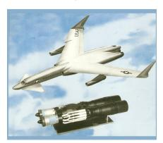
could not solve the excessive weight issues, the Direct Air Cycle by GE was simple, reliable, and doable. The prototype engine quickly exceeded the 100-hour full power requirement. Flight ready engines were developed and ready for testing.
